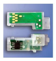
Notice there are three spring contacts on the underside of the ARC chip assembly. These will make contact with the OEM chip when installed as in the next step.
